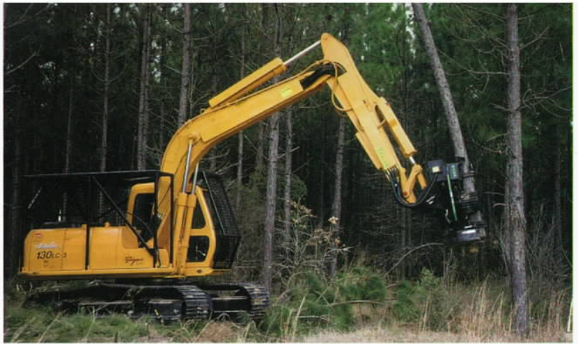
The HSG-140 and 160 allow a "controlled fall" rather than "free fall."
