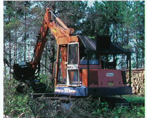
Aggressive roller design, large drive motors, and four delimit knives ensure quality delimiting, even under the toughest conditions.
